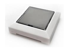
STM 550 provides an integrated NFC interface that can be used for device configuration and device commissioning. In addition, it contains an LRN button that can be used for simple commissioning tasks.
