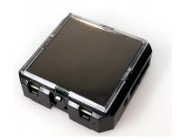
STM 550 provides an integrated NFC interface that can be used for device configuration and device commissioning. In addition, it contains an LRN button that can be used for simple commissioning tasks.
